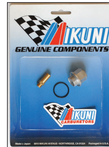
KHS-034 Main Jet Extender Kit Includes a Threaded Extension Tube for lowering the Main Jet into a deeper Long Float Bowl Drain Plug (TM32/41-1C) to reduce fuel starvation under full throttle and high performance applications. See listing Page 9
